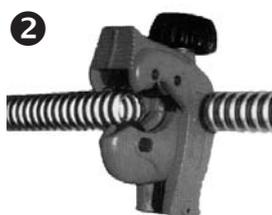
**2** Cut the measured tube portion **(2)** using the tube cutter contained in the toolbox. Try to make the cut as smooth as possible since it will influence the quality of the sealing surface.
