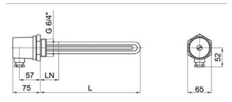
The elements feature a longer non-heating end (dimension LN) that permits their use for Regulus Thermal Stores with DHW.
