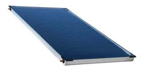
Flat plate solar collector of 1882 W output (at 1000 W/m<sup>2</sup> irradiance) designed for either portrait or landscape on-roof installation. A harp absorber with highly selective TiNOx surface is laser welded to copper tubing. The insulation consists of 40 mm mineral wool. Connection points are located laterally on the top and bottom.
