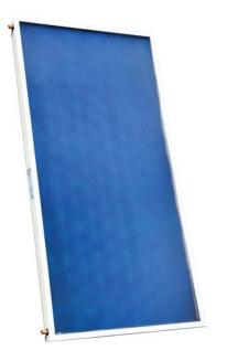
Flat plate collector of 1481 W output (at 1000 W/m<sup>2</sup> irradiance), designed for on-roof portrait installation. A harp absorber with highly selective TiNOx surface is laser welded to the copper pipes. The insulation consists of 40 mm mineral wool. Connections are located on both sides on the top and bottom.
