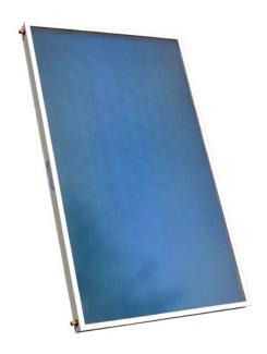
Flat plate collector of 1802 W output (at 1000 W/m² irradiance), designed for on-roof portrait installation. A harp absorber with highly selective TiNOx surface is laser welded to the copper pipes. The insulation consists of 40 mm mineral wool. Connections are located on both sides on the top and bottom.
