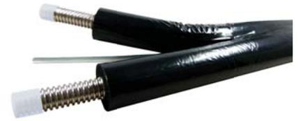
Two stainless steel pipes with silicone sensor cable (2x0.75mm<sup>2</sup>) in a double EPDM thermal insulation with PE coating that ensures enhanced protection against UV radiation. The pipes can be separated easily. They are marked to avoid interchanging the flow and return lines.
