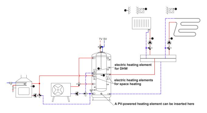
Hydraulic variant 2: Fireplace combined with a heat pump and a switched boiler (gas-fired, electric...)
