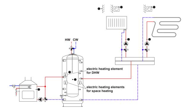
Hydraulic variant 2: Fireplace combined with a switched boiler (gas fired, electric fired..)
