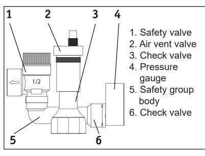
Mount the safety group as close to the boiler as possible and above the highest level of the heating source.
