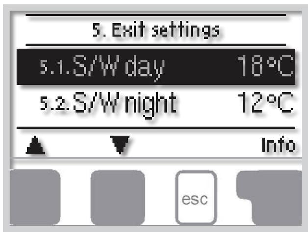
The necessary basic settings required for the control function of the heating circuit are made in menu „5. Settings HC”.
