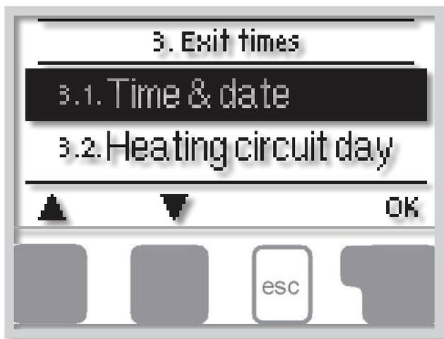
Menu „3. Times” is used to set the time, date and operating times for the heating circuit.
