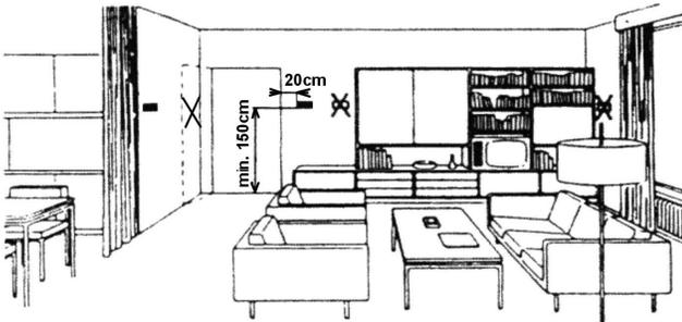
The thermostat is designed for indoors usage only. It should be placed on an inner wall about 150 cm above the floor, into a suitable space where changes in the room temperature can be registered thanks to freely circulating air.
