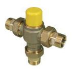
DHW thermostatic mixing valve for solar systems, outer thread with coupler, check valve and strainer, temperature fixed at 48 °C
